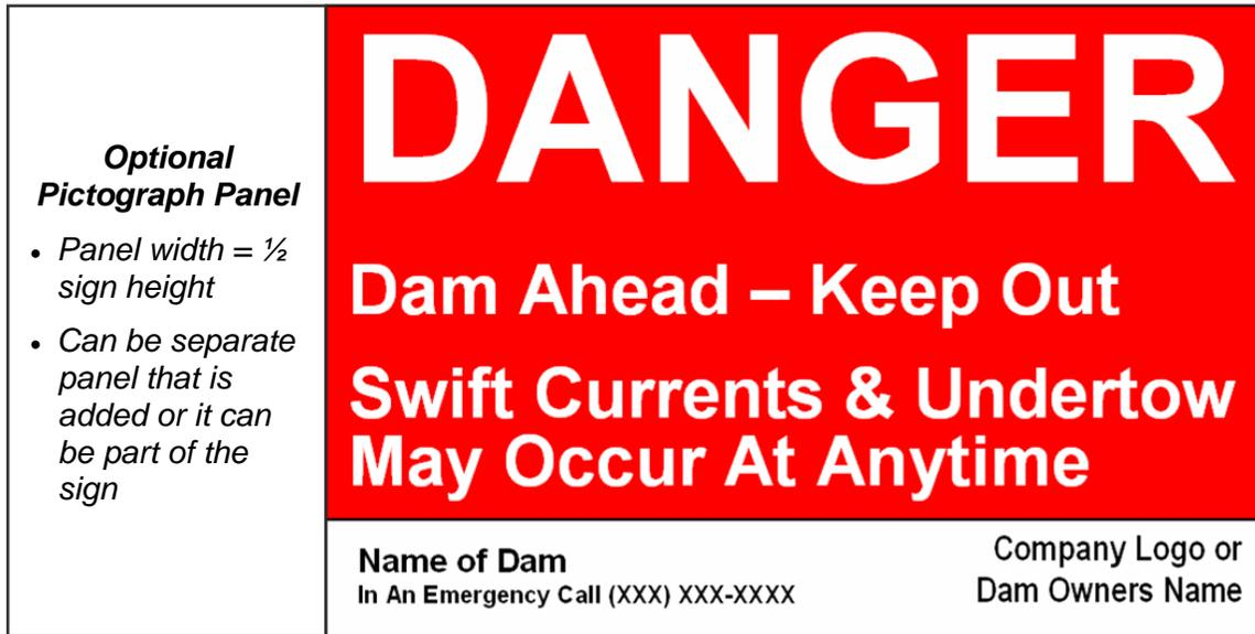
Figure C.8: Warning Sign - Dam Upstream
